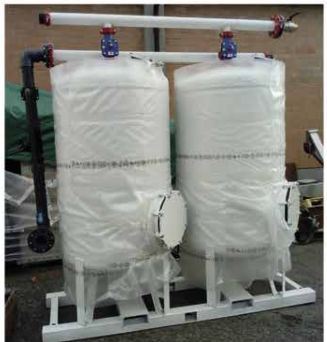
Tertiary water treatment - filtration
